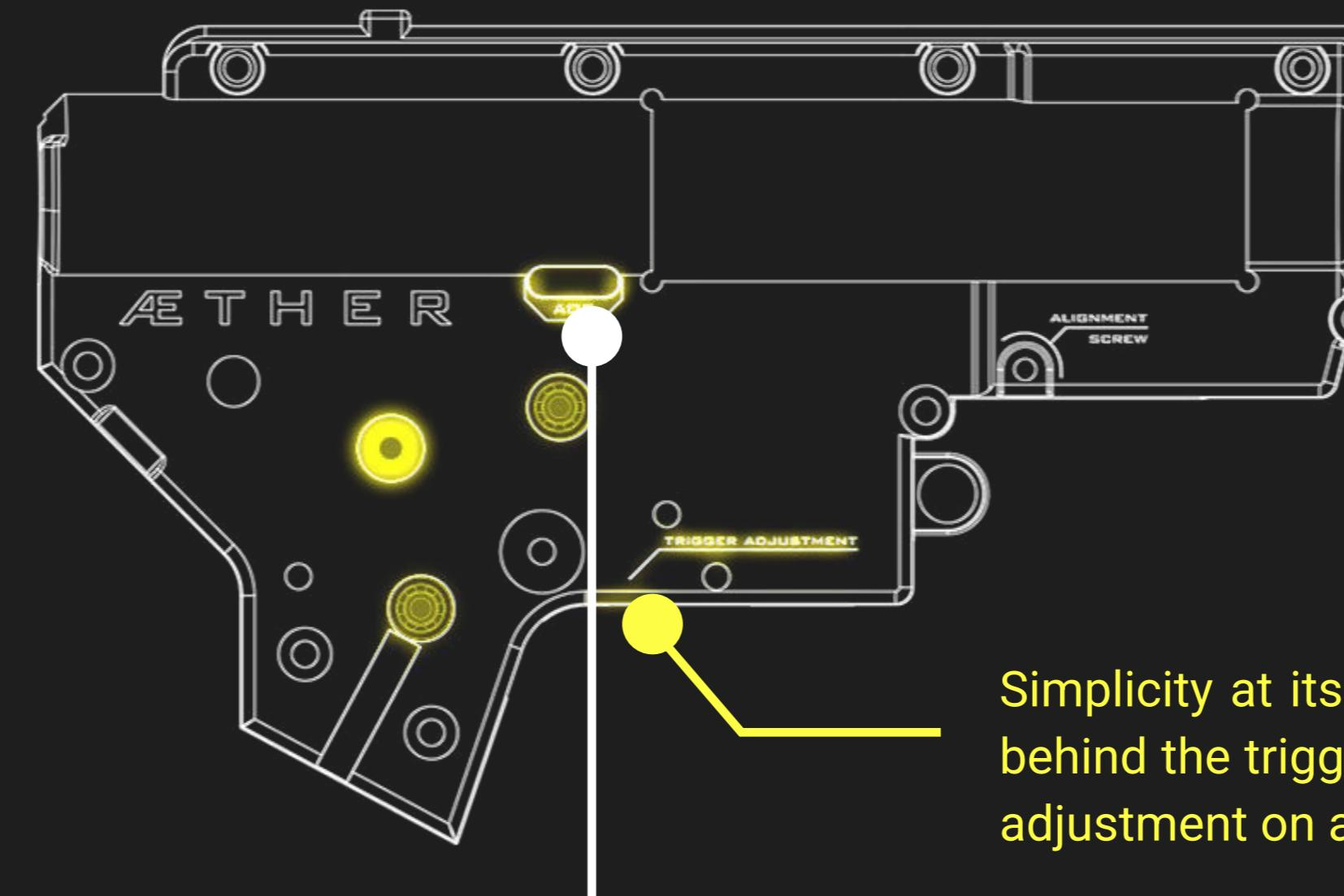
Simplicity at its best! A small screw located behind the trigger axis allows for pre-tension adjustment on any V2 gearbox trigger.
